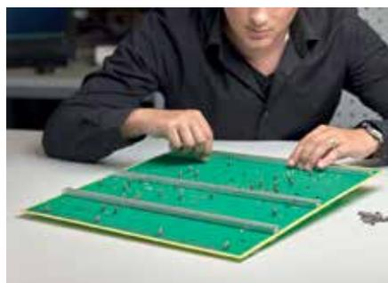
Mounting of reinforcement beams between connector and spacer board
