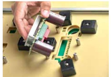
Due to the concept of the TEST-OK Modules, it is possible to test different types of UUTs with high components on both sides
